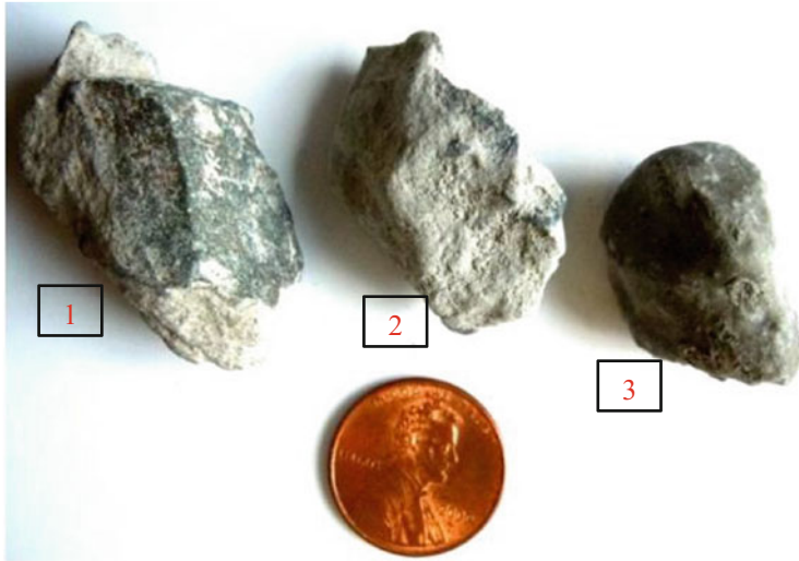
Fig. 8.22 Untreated (1) R_0 and treated RA samples (2) R_1 (3) R_2 (Zhang et al. 2016)
