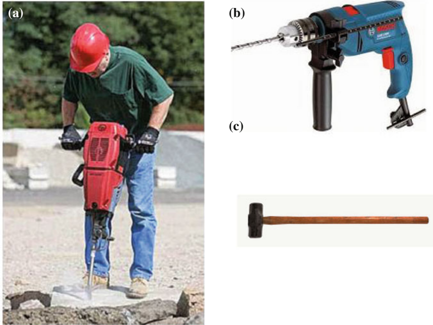
Fig. 2.1 Manual tools (a) Jack hammer (b) Drill and (c) Sledge hammer (Adopted from Prakash 2014)
